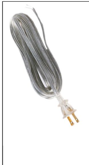
*All SPT2 15' with 1-15P male plug, twist & tinned, hanked
